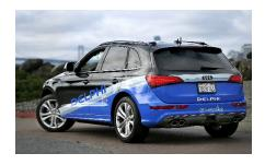
the road around it. The SUV is expected to maneuver around bicyclists and pedestrians, navigate four-way intersections and merge with highway traffic.
